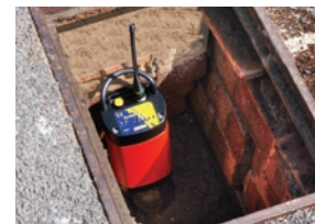
Internal accelerometer connects direct to pipe
